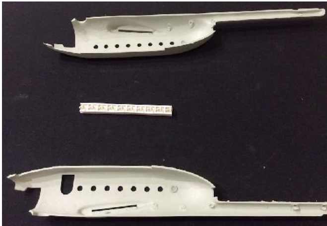
Forward door and slot cut for undercarriage bay from fuselage. Rear portholes filled
