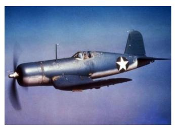
To accommodate such a large diameter prop, a novel approach was adopted by the design team which also went a long way to reducing any weakness in the undercarriage of the machine. Of course this was the so called gull wing, it's shape reduced air resistance by virtue of the fact that the wing was attached to the fuselage at the optimum angle. One prototype was ordered and first flew in
